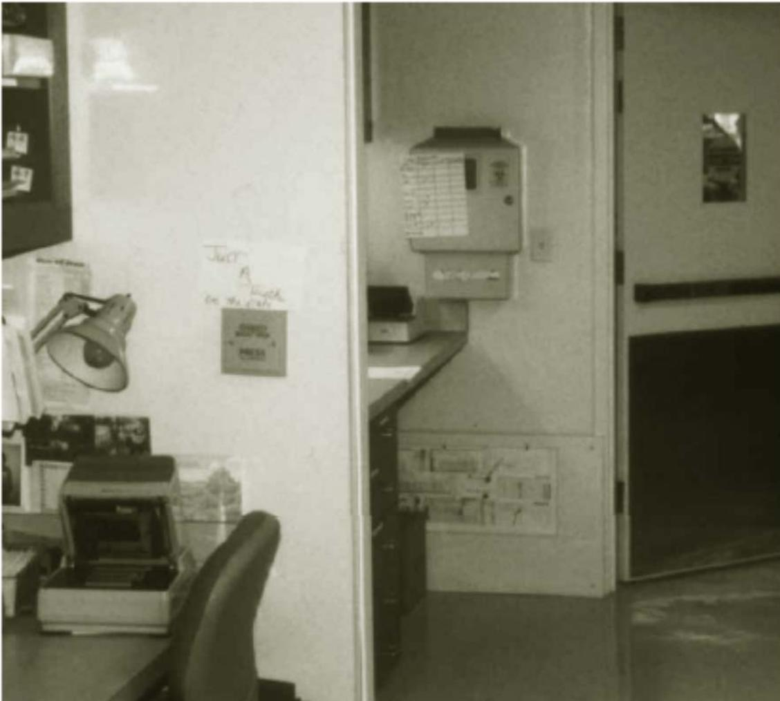
**Figure 10 depicts how the plate to open the doors has been relocated to approximately 8 feet in front of the doors. This allows a person pushing a stretcher to operate the door control without having to leave the patient**
