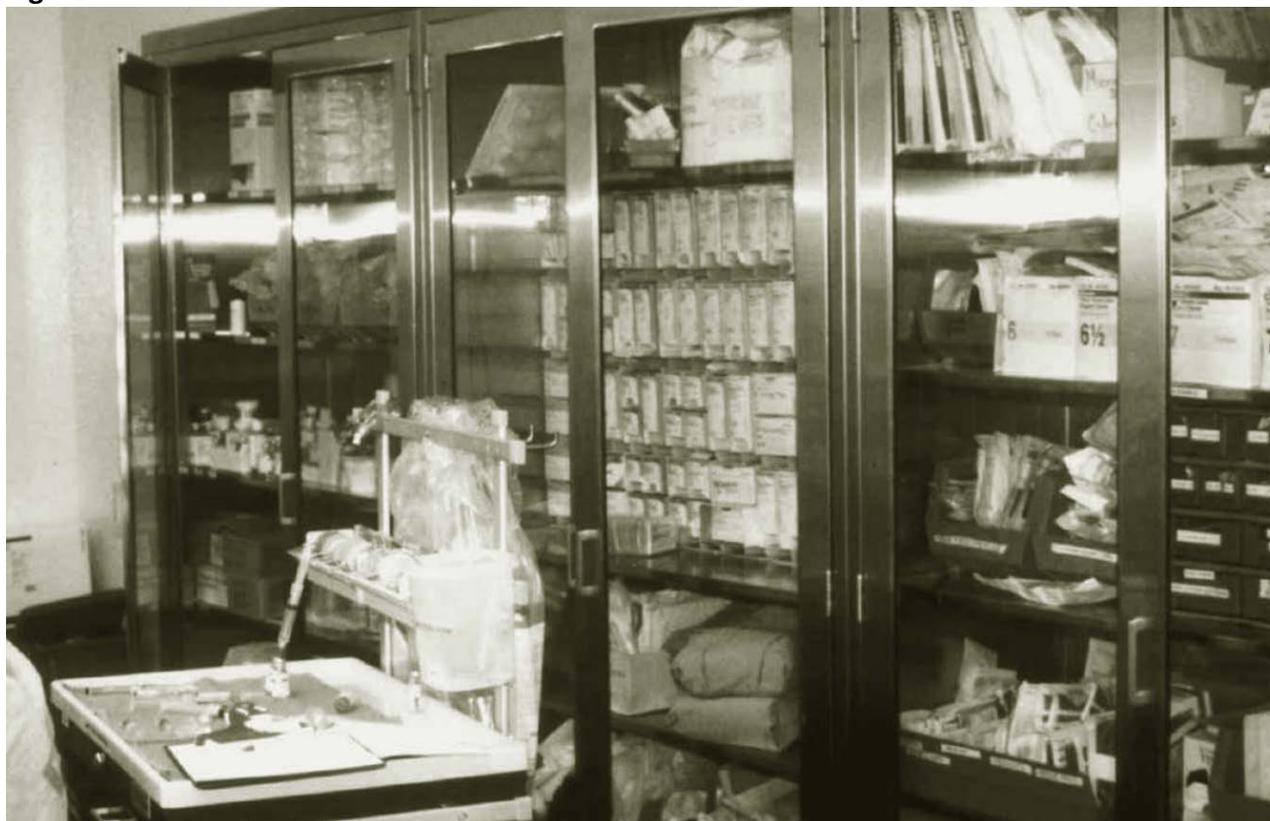
**Figure 8 depicts a room that has the anesthesia supply cart located in front of the storage cabinets, making it difficult for the nursing staff to access the supplies. The room should have been designed so that movable equipment was kept away from the supply cabinets.**
