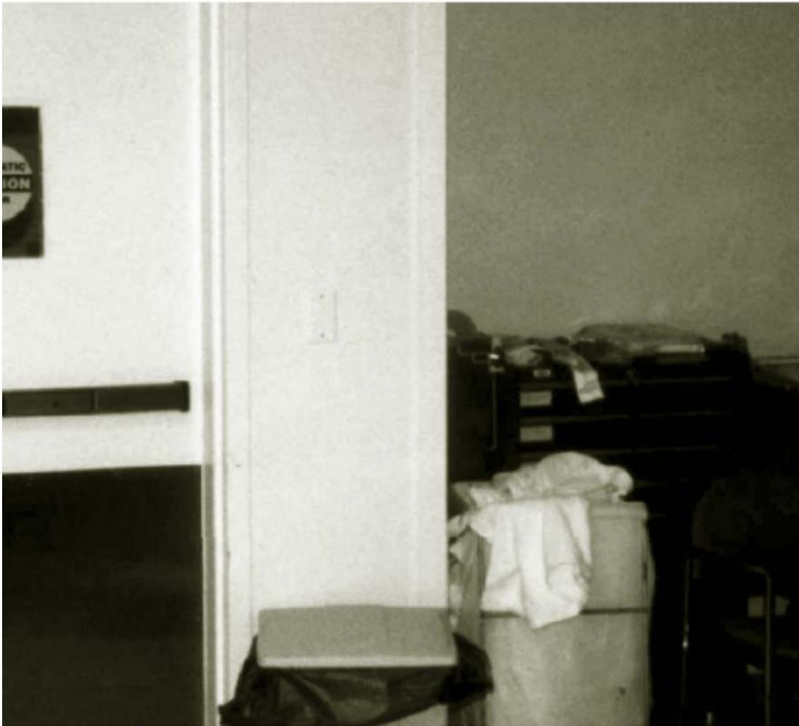
Figure 9 depicts automatic doors leading from the preoperative holding room into the OR that require a plate to be pressed in order for the doors to open. The plate was originally located on the wall next to the doors (note the blank cover plate to the right of the doors). This made it impossible for a person pushing a stretcher to open the doors.
